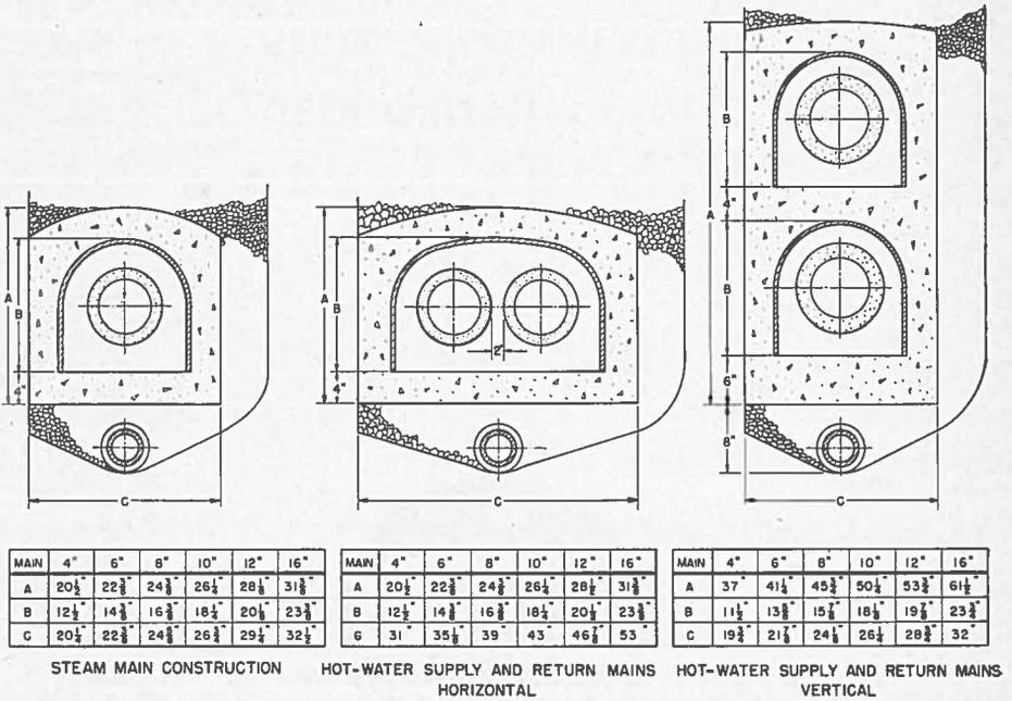
FIG. 4—Comparison of Conduit Cross Sections for District Heating by Steam and High-Pressure, High-Temperature Hot Water
