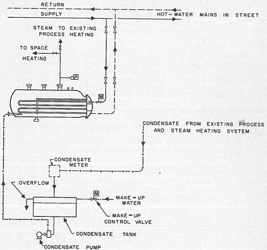
FIG. 2—Heat Exchanger and Piping Arrangement Where High-Temperature, High-Pressure Water Is Available in the Street Mains to Provide Steam for Space Heating and Process Use
