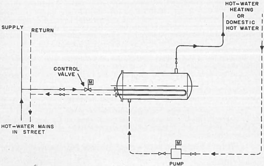
FIG. 1—Heat Exchanger and Piping Arrangement Where High-Temperature, High-Pressure Water Is Available in the Street Mains to Provide Low-Pressure Hot Water for Space Heating and Process Use
