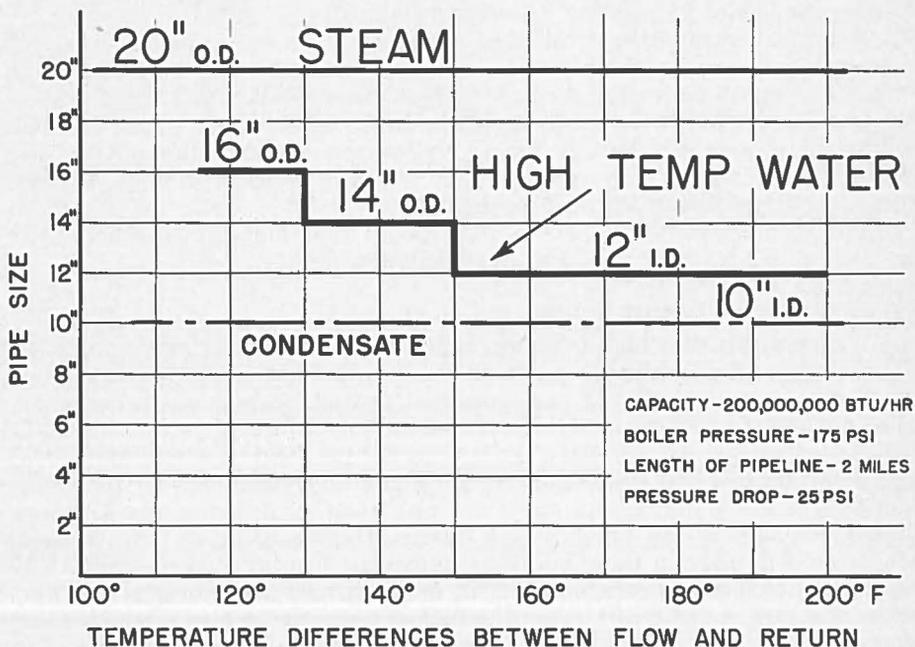
FIG. 3—Comparison Between Pipe Sizes for Steam and Hot Water for Transmitting 200,000,000 Btu per Hour Under the Conditions Stated<sup>1</sup>
