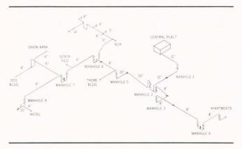
FIG. 1 - Isometric drawing of the high-temperature water system.
