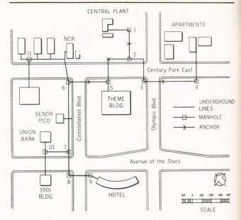
FIG. 2 - Plan view of Century City piping system.
