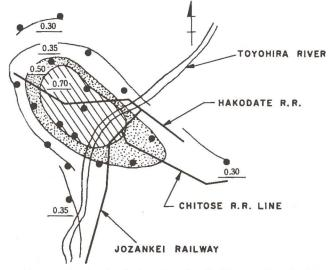
FIG. 2 — Density distribution of sulfur dioxide gas after district heating.
