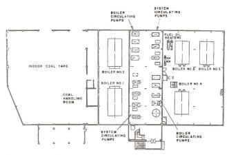
FIG. 5 — Plan of central heating station.
