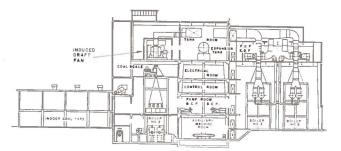
FIG. 6 - Section of the central heating station.
