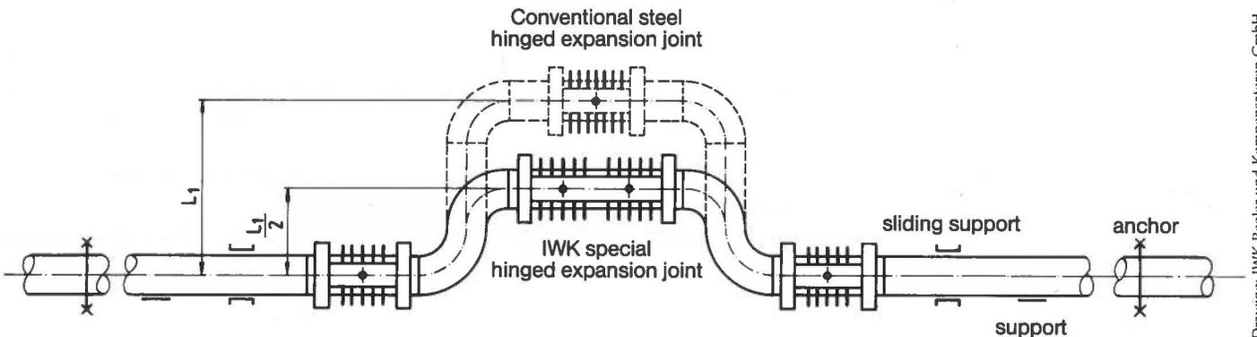
*Three-hinge U-loop systems represent a customary method of taking up thermal expansion district heating lines. A new, special hinged expansion joint has been developed with which angular rotation is doubled and the projection (L1) thus halved.*
