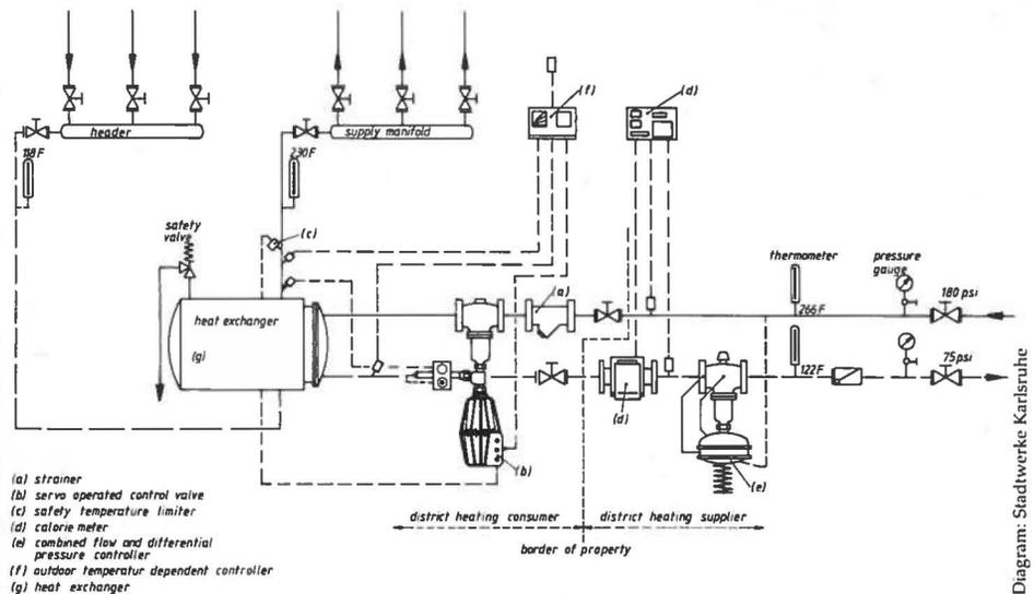
Circuit diagram of building connection. Including the necessary metering and control equipment and the heat exchanger.
