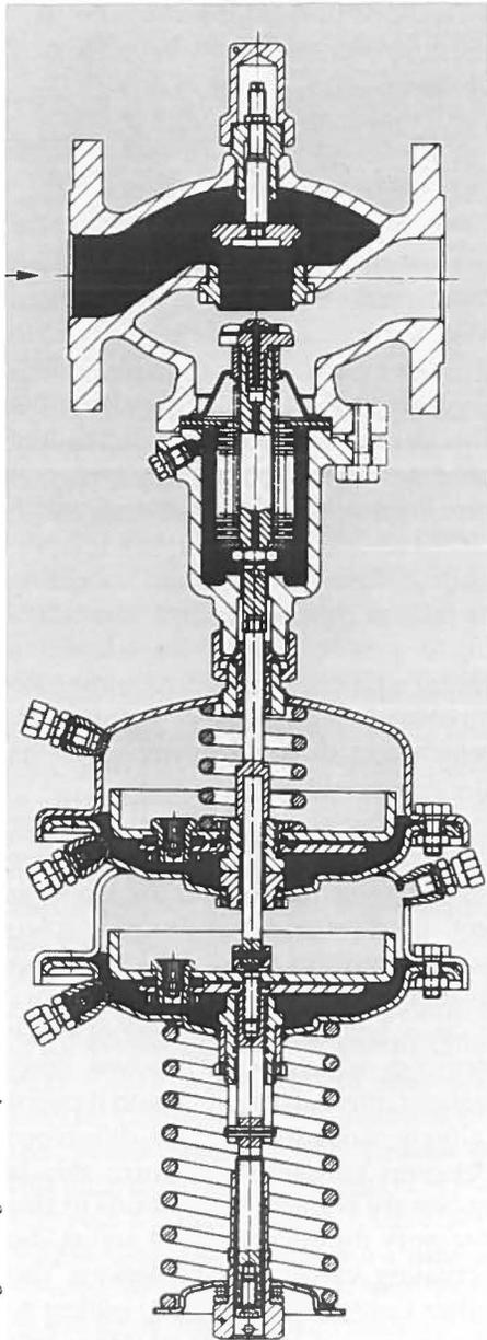
*Cross section through a flow and differential pressure controller. It maintains the pressure difference between supply and return flows constant and limits the heating water flow volume to an adjustable maximum value.*
