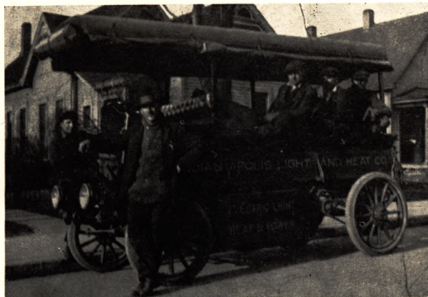
The first two line trucks in Indianapolis electric service were battery-powered Waverlies, which were relied on for faster runs than horse-drawn wagons could make for storm trouble or other emergencies. In the line crew shown on one of these trucks, in 1916, were (left to right) Tona Heishman, foreman and chauffeur; Charles Hurst, Levi Collins, Basil Clark and Orvel Poe.
