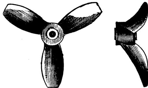
In the case of a torpedo boat, 58 ft. long, the substitution of one of Mr. Thornycroft's screws for an Admiralty screw with the corners cut off was found to increase the speed from 16½ to 17½ miles per hour, while in Mr. Perkins' small steam yacht, the Emily, the application of one of these screws in place of Griffith's, raised the speed about one knot in seven. Similar results have also been obtained in other instances, the speed being increased and the vibration greatly reduced.—*Engineering.*
