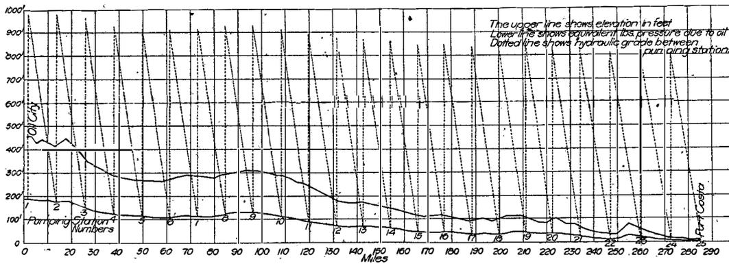
Profile of Rifled Pipe Line for Pumping Heavy Oils.
