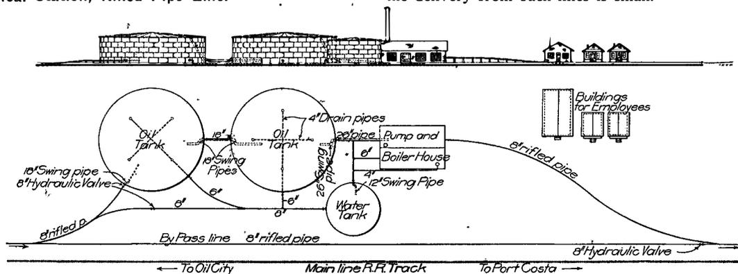
Arrangement of a Typical One of Twenty-three Pumping Stations.
