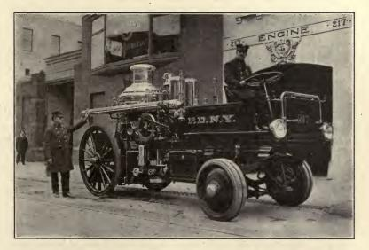
Self-Propelled Steam Fire-Engine, Period of 1917
