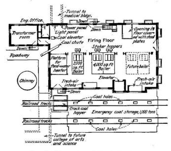
Fig. 5-Floor plan of the boiler house
