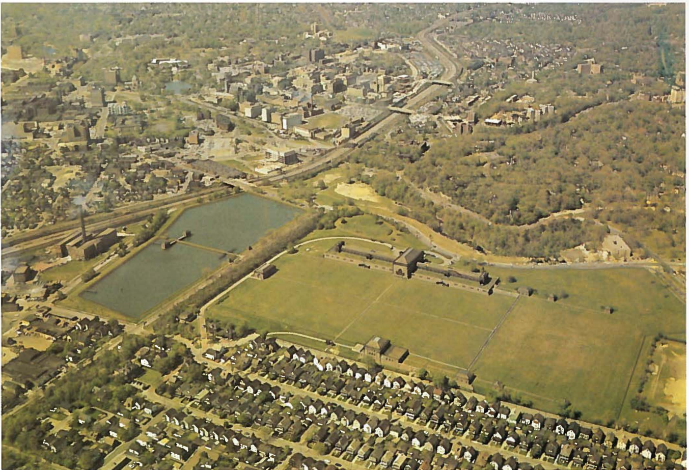
Baldwin Filtration Plant and Fairmount Pumping Station complex includes a covered reservoir (under lawn) believed to be the world's largest. When an electrification program is completed, treatment capacity will be 200 million gallons daily.
