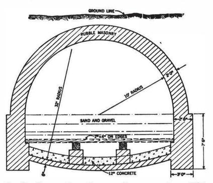
FIG. 49. UPWARD-FLOW FILTER AT BURLINGTON, IOWA, 1878 Designed and built by T. N. Boutelle, Engineer;  $20 \times 130$  ft. in plan (From blueprint supplied by Frank Lawlor, Supt., Burlington Water Works)
