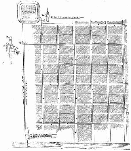
Fig 1. Reversing Apparatus. B. Back Pressure Valve. C. Operating Cylinder. -0 Fire Hydrants. D. Safety Valve.
