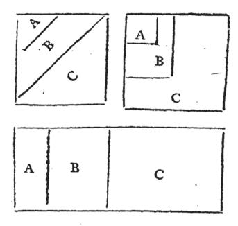
The forms in the margin may convey an idea of plans of three vessels supposed to be made of one or other of the said materials, wherein the space A, represents the bottomless tube, which is to receive the turbid water from the ball cock, and discharge the air from the grateing, &c. under it.
